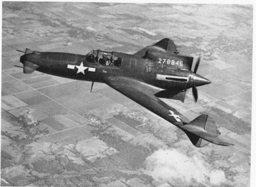
The fast and highly maneuverable Curtiss (XP-55) Ascender that literally hurls itself through the air with power produced by 1275 horsepower engine driving a propeller in the rear. It is a low-wing, all metal, "tail first" single engine pusher-type experimental aircraft developed by the Curtiss-Wright Corporation for the Army. Scovill-made parts have been built into this experimental development of one of the most unusual plane designs.
